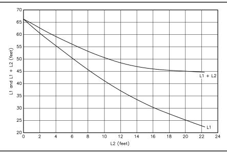
Fig 4—Effect of top loading on radial length.
